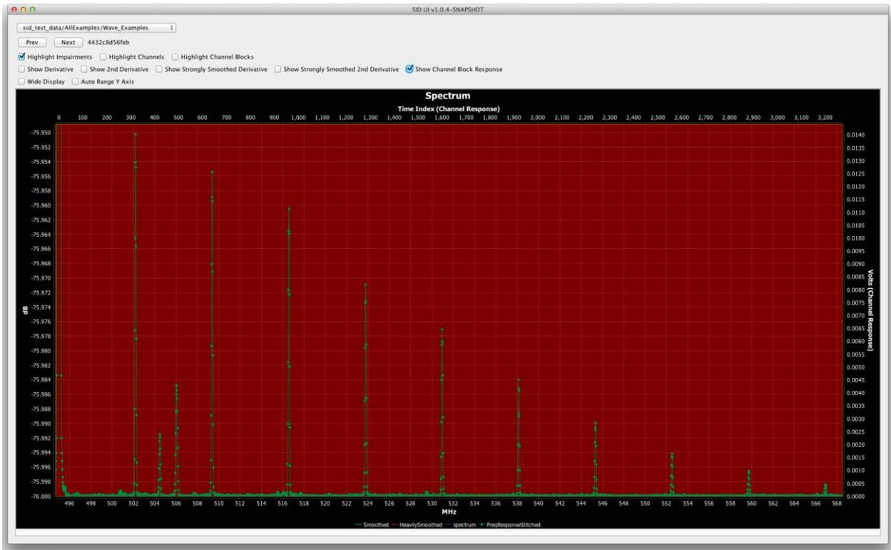
Figure 2 Screenshot of SID zoomed in on the time domain showing the channel comb and the 2 wave impulses
