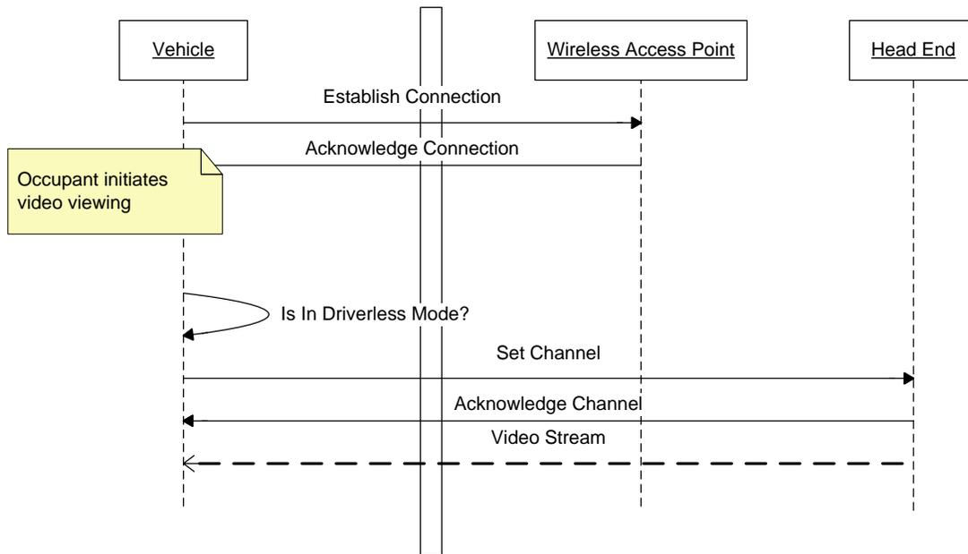
**Figure 1 Driverless Video Communications**
