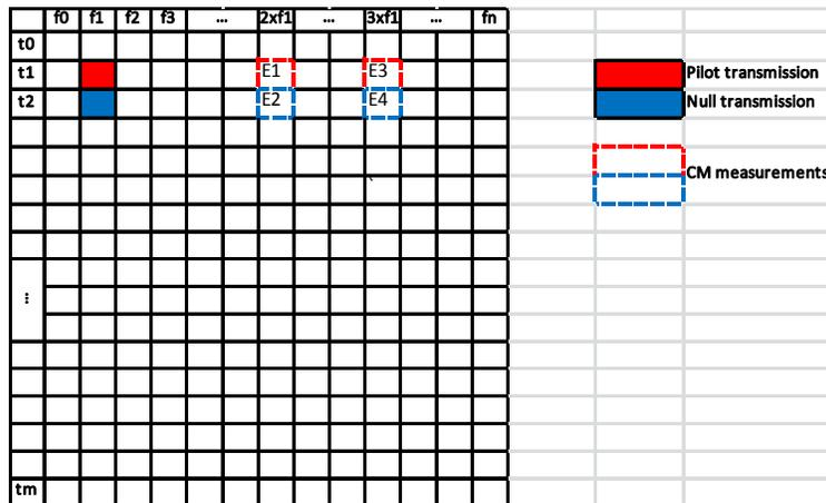
A potential addition to the invention would be the incorporation of two tone tests by having two pilots transmitted at the same time separated by a certain frequency gap. The measurement would be conducted in the intermodulation expected frequencies. This would allow intermodulation distortion testing.
