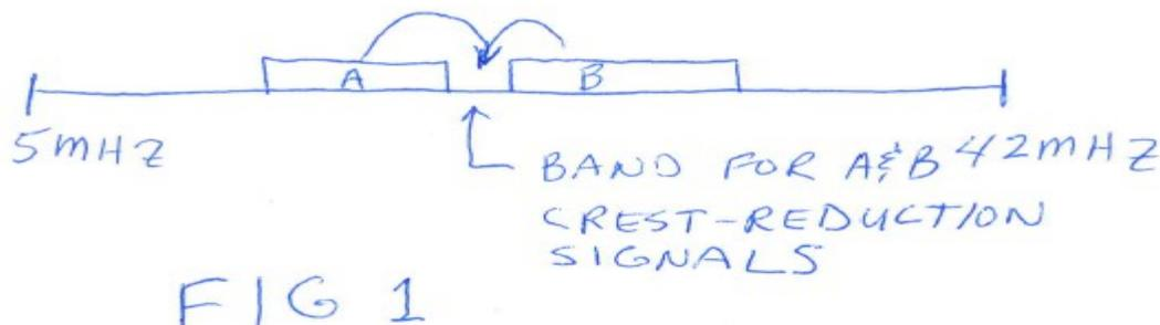
In a basic implementation, a number of subcarriers will be left vacant in between two spectral blocks that require PAPR reduction. PAPR reduction will be required when a CM's transmit power is near its maximum.
