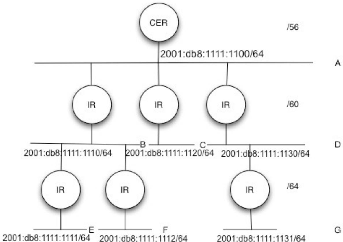
Our invention is an enhancement to this network architecture. Assuming that multiple IP prefixes (e.g. IPv6 ULA, IPv6 GUA, and IPv4) are distributed via prefix delegation in a three level hierarchy using four bits per level, there will be 8 bits in common at every
