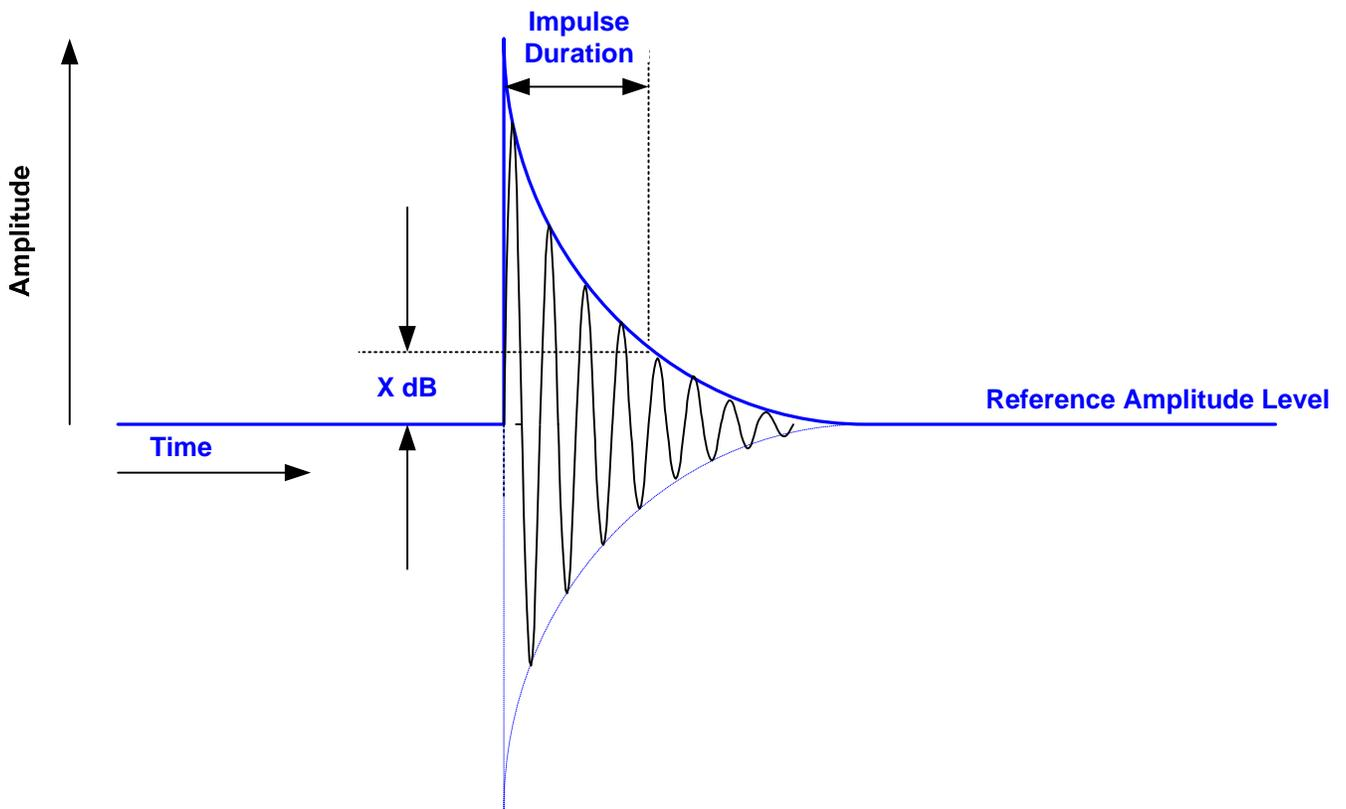
*Figure 2 – Time Domain Representation of Typical Impulse*
