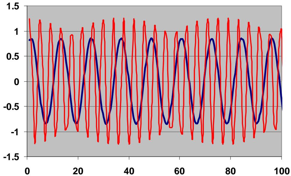
Figure 7 Time view of narrowband interferers affected by micro-reflection
