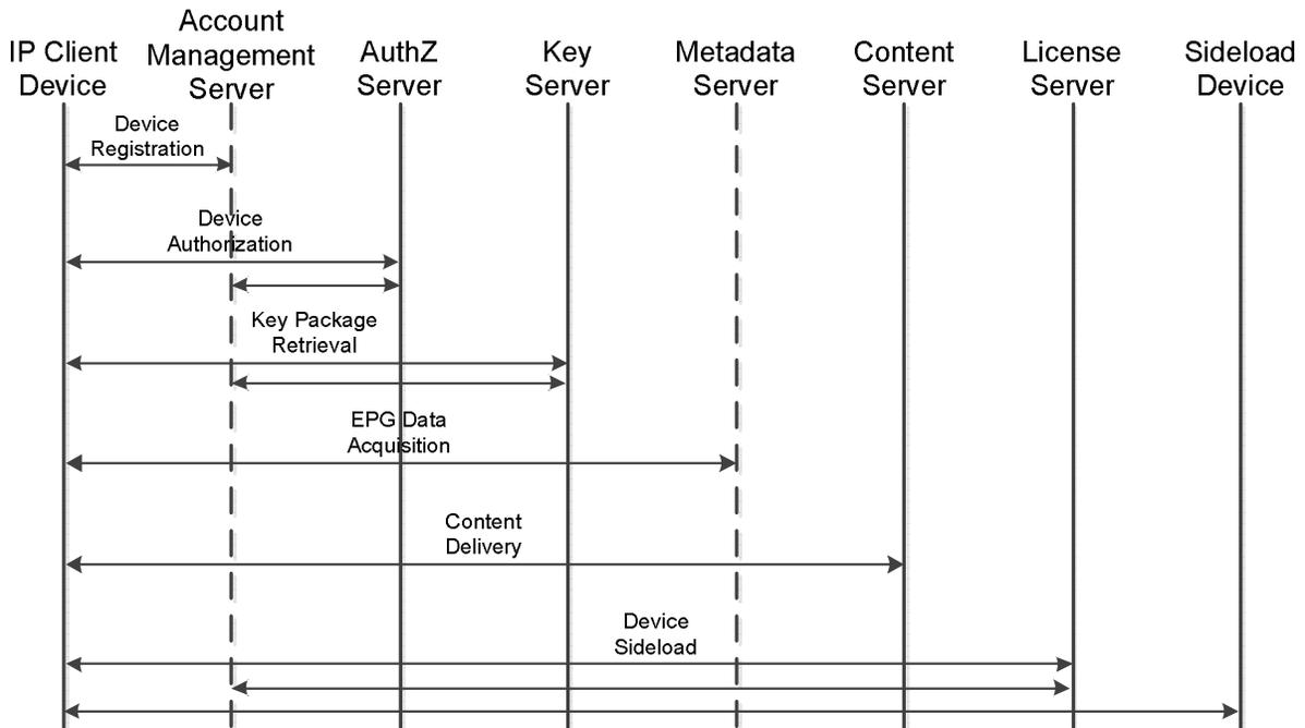
Figure 3. System Component Interaction
