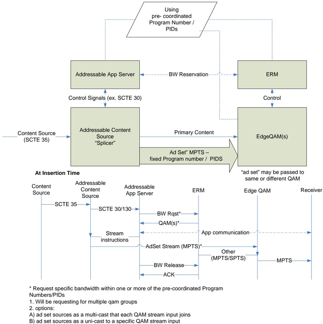
**Figure 0-8 -Digital Program Insertion Diagram**
