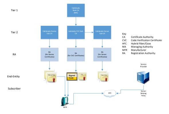
Figure 1: CableLabs PKI Architecture
