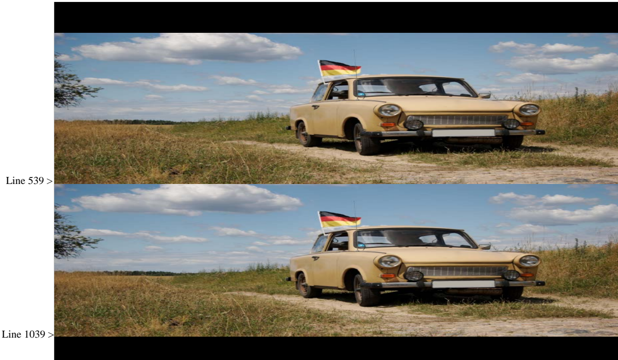
Figure 9 - TaB formatting with incorrect letterbox alignment
